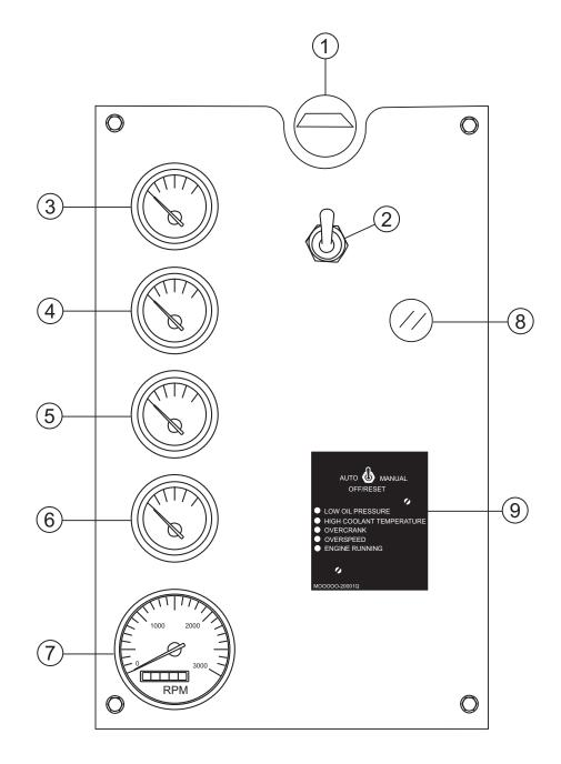
Figure 7. Engine Operating Panel
